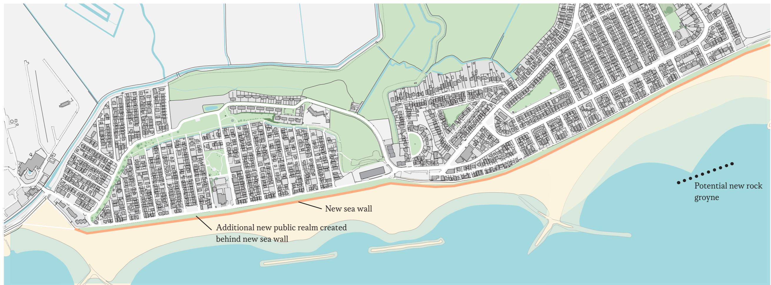
Fig. C22. Map showing line of new sea of wall proposed under Option B, and location of potential additional rock groyne
