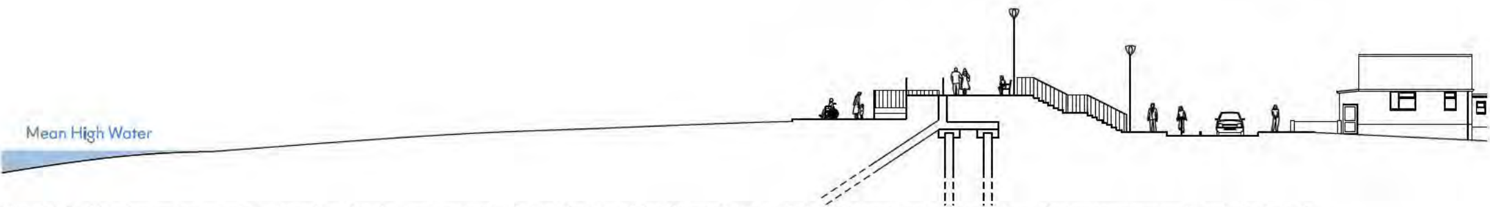
Fig. 66. Indicative cross-section showing the design framework for the Brooklands seafront and the distance to high water at the narrowest point of the beach.
