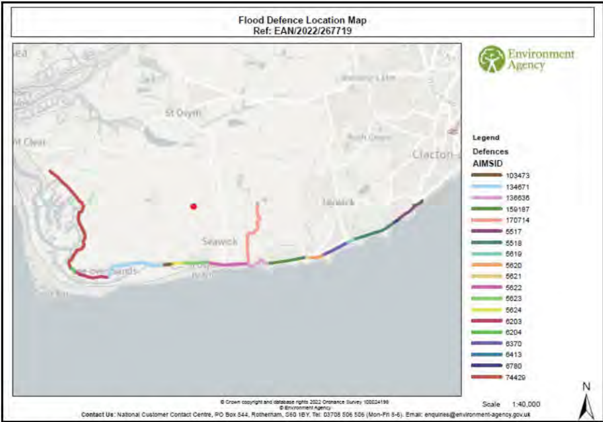
Fig. 30. Extent of the flood 'cell' in which Jaywick Sands is located. Upgrades to all the defences shown would be required to continue to protect Jaywick Sands in the future. Source: Jaywick SFRA, 2023.
