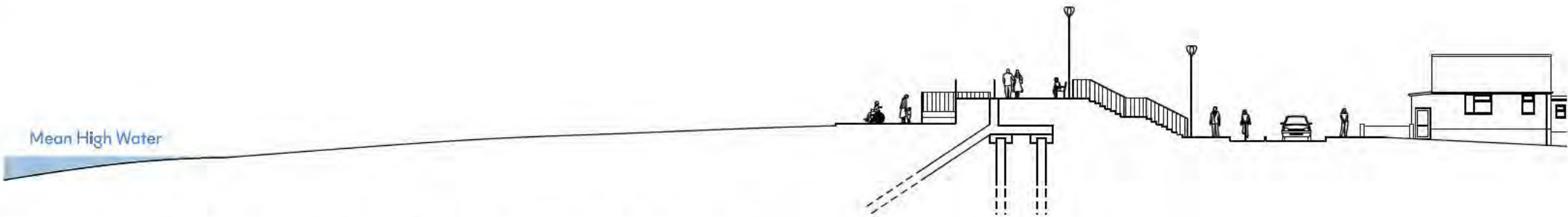
Fig. C27. Option B - indicative section through beach and sea wall at Brooklands.
