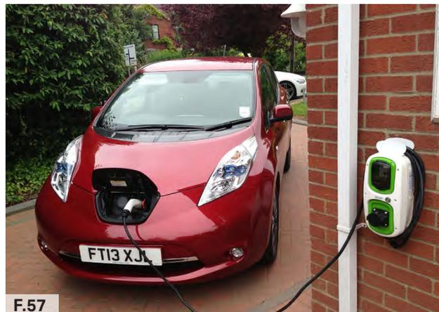
**Figure 57:** Examples of off-street mounted car charging points.
