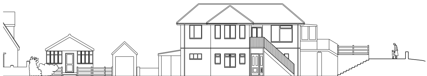
Fig. 37. Side elevation / cross-section of seafront plot and level change to promenade
