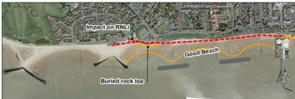
Figure 6-6: Zone A Detached breakwater layout
