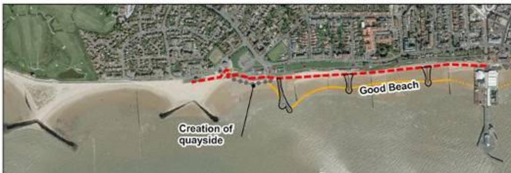
Figure 6-7: Zone A fishtail breakwater indicative layout
