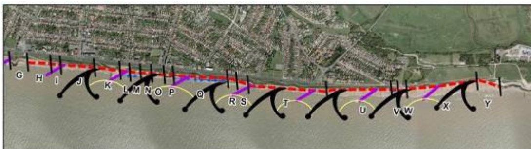
Figure 6-19: Zone C fishtail breakwater indicative layout
